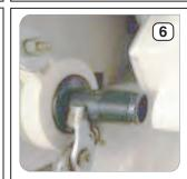
Grab drain tube with a plier or similar tool and put into housing until it hits the stop about 1-1/4" in depth.
