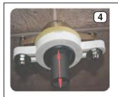
Lubricate drain tube and insert into coupler. Run in and out until this can be done easily.
