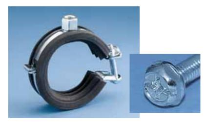
The CADDY® SUPERFIX 454 is an easy-to-close pipe clamp that works on steel and copper pipes from 1/4" (12 mm) to 4" (114 mm). A unique hinged design eliminates the need to disassemble the clamp prior to installation and allows the installer to close the pipe clamp with one hand without turning a screw. Once the pipe is installed, simply tighten the screw to secure the pipe in place.
