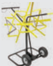
Uncoiler - Not for center pull coil, 1" tubing or larger, Viega FostaPEX components Movable metal frame, (2) coil hubs, tube guide Note Max. coil size for 3/8" and 1/2" tubing is 1000 ft. Max. coil size for 3/4" tubing is 500 ft. Model V5061
