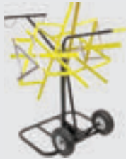
Uncoiler - Not for center pull coil, 1" tubing or larger, Viega FostaPEX components Movable metal frame, (2) coil hubs, tube guide Note Max. coil size for 3/8" and 1/2" tubing is 1000 ft. Max. coil size for 3/4" tubing is 500 ft. Model V5061
