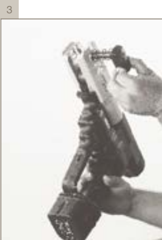
3 - Creating the lugs for Ø 3", Ø 4" or Ø 6" cut pipe Open the retaining pin at the front of the machine by pressing the jaw release button
