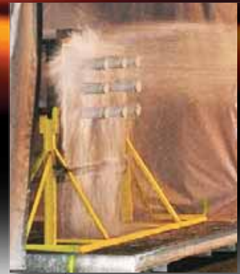
Hose stream test
