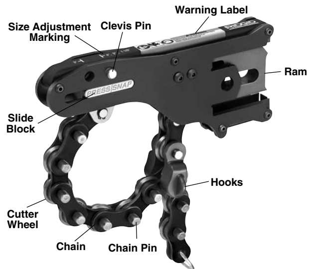
Figure 1 – Press Snap Soil Pipe Cutter
