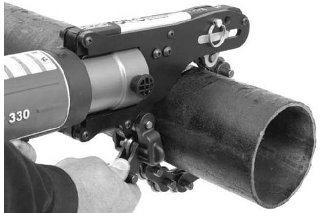
Figure 4 – Wrapping Chain Around Pipe
