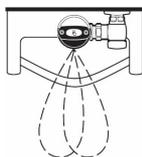
3. When the user steps away from the Sensor, the Sensor initiates an electrical signal that operates the Solenoid. This initiates the flushing cycle to flush the fixture. The Circuit then automatically resets and is ready for the next user.
